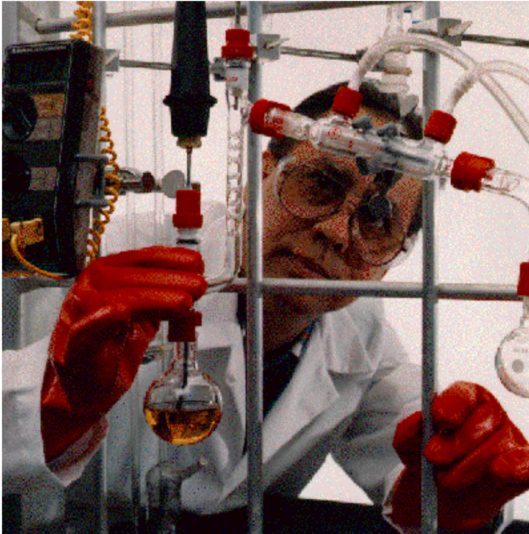
Fig. 1. An engineering technologist sets up an apparatus in which PCB-contaminated liquid will be exposed to chemicals which remove the chlorine from the compound, transforming the PCBs into non-regulated chemicals.
